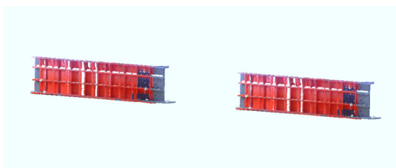
Figure 10. Two steel beams before splicing
